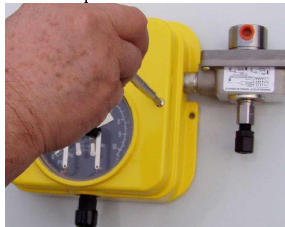
Fig. 10 Close and secure with front screws to insure proper sealing and protection from environment.
