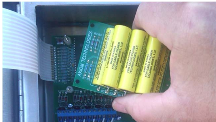
Fig. 6 Align the battery module with threaded studs and push it in place gently. The "Axiom Technologies" printing on the module is to be on the left.
